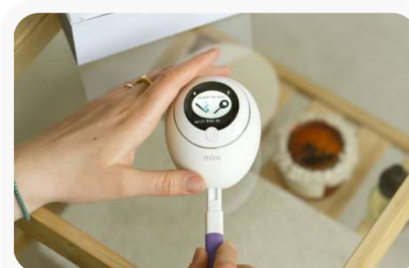
Step 2 Insert the wand into the Mira Analyzer.
